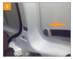
Insert the counterplate from the side up to the position and using the template from the outside (using the 9 holes made) center the counterplate and tighten. Take care to avoid detaching the counterplate from the drive rod before fixing.
