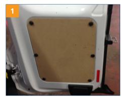
Remove the paneling of the two doors of the rear door. Apply the drilling template. In particular, the longitudinal axis of the shell is 48 cm from the lower edge of the door. Align the vertical axis (dash line) with the edge of the tailgate. Mark the 9 mm holes.\*
