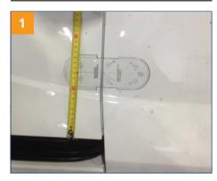
Remove the side door and side panel paneling. Apply the drilling template. In particular the longitudinal axis of the shell at 13 cm from the sliding guide seat. Mark the 9 mm holes.\* Combine the counterplate with a rod / slab (with a thickness of less than 3 mm) in steel or plastic, using gummed paper (or other adhesive tape) to have good handling and stiffness.
