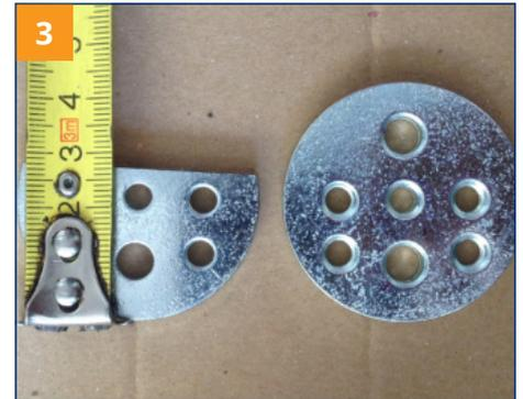
Cut the striker plate as shown next (approx. 3cm). In this way the same will fit perfectly into the existing internal site. Check that there is no interference with the standard lock. **Proceed with the steps according to the product technical information.**
