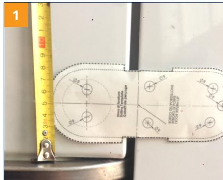
Remove the panels from the sliding door and the side part. Apply the drilling template. In particular, the longitudinal axis of the body lock is at 5 cm from the upper side of the sliding side. Mark holes 9 mm.\*
