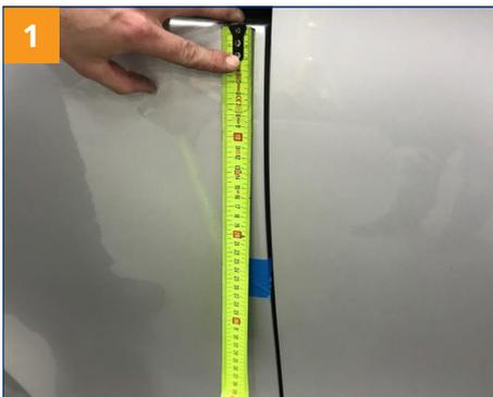
Remove the panels of the door and the side part. Apply the drilling template. The longitudinal axis of the outer shell is 23 cm from the lower part of the side rail (see picture). Align the vertical axis (dash line point) to the edge of the tailgate.
