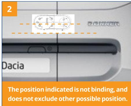
Align the vertical axis (dash line point) to the edge of the tailgate. Mark the 4 holes of 9 mm extremes.\*
