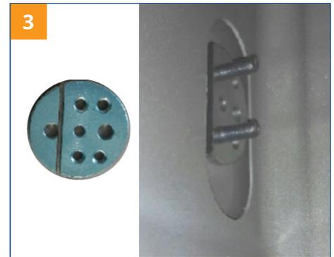
Cut the backplate as shown in picture. This way, it will be possible to insert it inside a seat created inside the door. **Proceed with the steps according to the product technical information.**
