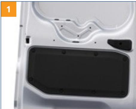
Remove the panels from the sliding door and the side part. Apply the drilling template. In particular, the longitudinal axis of the body lock is at 4cm from the bended sheet metal over the door handle (see picture at right).
